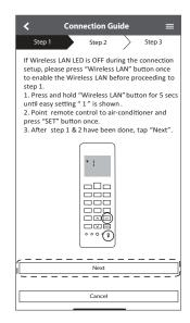
3. Ensure Wireless LAN LED is ON. Press and hold the Wireless LAN so button for 5 seconds until "1" is shown on the remote control and press st pointing to the air conditioner.
