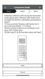
3. Ensure Wireless LAN LED is ON. Press and hold the Wireless LAN 🕏 button for 5 seconds until "1" is shown on the remote control and press 💷 pointing to the air conditioner.
