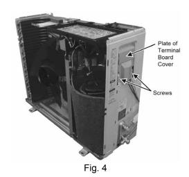
6 Remove the Control Board.
