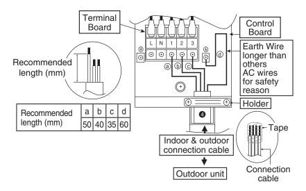
6 Secure the connection cable onto the control board with the holder.
