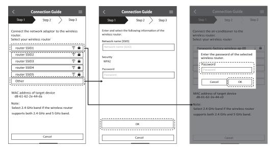
4. Select the SSID of your wireless router. Enter the password to connect the air conditioner to the wireless router.
