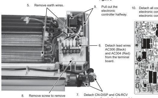
Detach all connectors as labelled from the electronic controller. Then pull out the electronic controller gently.
