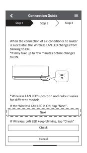
When the connection of air conditioner to router is successful, the Wireless LAN LED changed from blinking to ON.
