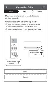
Ensure Wireless LAN LED is ON. point the remote control to air conditioner and press Wireless LAN putton until the Wireless LAN LED changed to blinking.
